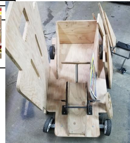
Build Kit Plus parts with resulting cart
